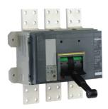
Circuit breaker, PowerPacT R, 3000A, 3 pole, 600VAC, 18kA, busbar, Micrologic 5.0, 100%
